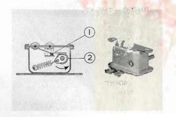
2. See that the rotating cam is correctly timed to the accelerator pedal.
