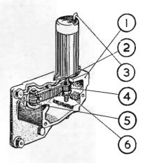
Note.—A simple way to energise the solenoid is to break the snap connector at the Solenoid terminal and connect with a short lead direct to battery negative.
