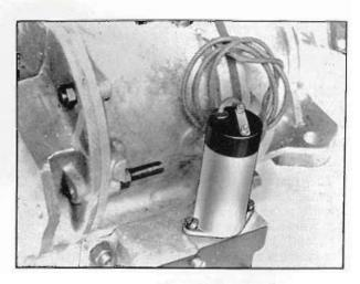
simply to open and close the hydraulic actuating valve for the overdrive gear change.
