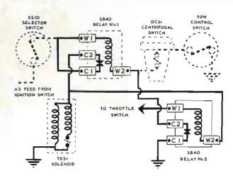
With the throttle more than one fifth open the switch will also be open and the car will return to normal gear until the centrifugal switch contacts again close and changes it back into overdrive.
