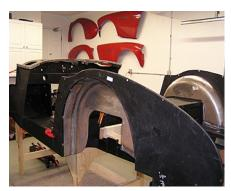
The welding of rear bumper outriggers, emergency brake supports, front motor mounts, firewall and radiator supports, etc. is now complete. These along with the temporary affixing of other tub components is also complete. The last photo illustrates the rear shroud in place, albeit temporary, this tells me that the progress is in the right direction. My current problem is some sheet metal welding difficulties with the 19 gauge tub pieces. For the present -cheers!
