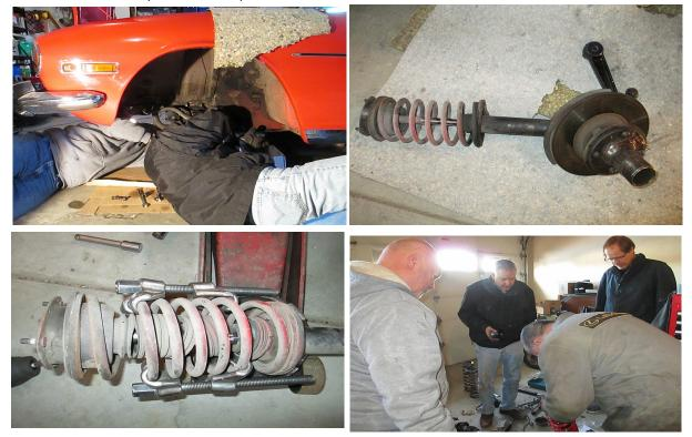
Bob remarked the old struts had been rather roughly put in place in the past, and one strut had completely broken down. It was a job worth doing, and now a safer 'old Brit' is back on the road.
