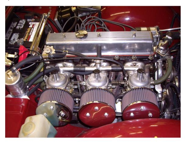
The engine ran strongly. The only things I did was to remove all the original emission system equipment (that did nothing to restrict pollutants anyway). I installed K & N filters and an oil separator to prevent excess oil passing through the carburetors from the PCV valve. (it's the small round tank on the extreme left side of the photo above).
