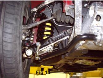
Finally I wanted to stiffen up the steering rack mounts as the stock rubber bushings promoted a slightly sloppy feel at the steering wheel. Instead of replacing the stock bushings I installed solid aluminum brackets that eliminate any play or give at the mounting points.
