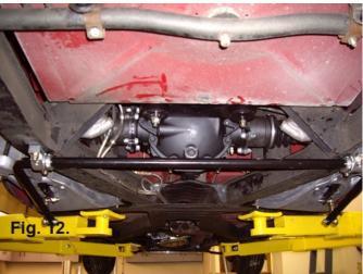
Once the springs and shocks are in place, the new hubs and CV axles (**Fig. 11**) were installed and bolted up to the diff. and the trailing arm housing. I had to check for any interference between the CV joints and the inner walls of the trailing arm housing as this is a pretty tight fit.
