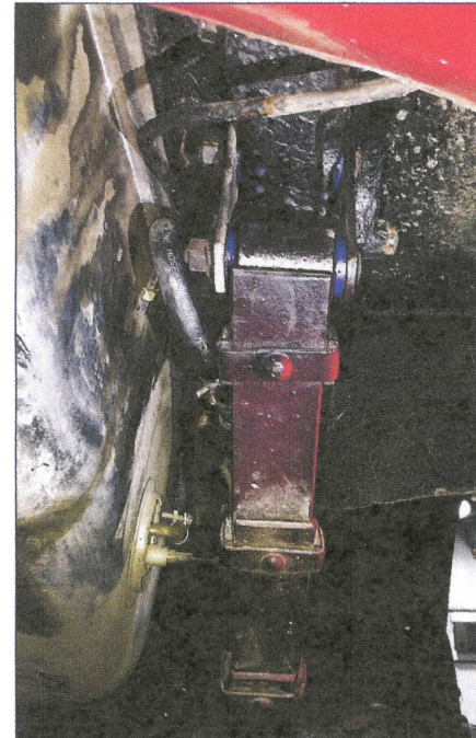
Polyurethane bushes installed on the leaf springs.
