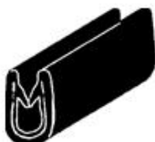
T/FAST 100 BLK or LT.GREY (flange 1.587mm - 4.762mm)
