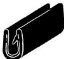
T/FAST 101 BLK or WHITE (flange 3.967mm - 4.762mm)
