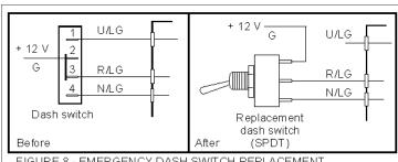
FIGURE 8 - EMERGENCY DASH SWITCH REPLACEMENT
